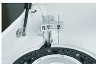
Washing Probe Independent 3 -step washing system.
