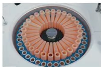
Reagent Tray Refrigerated tray with independent switch.
